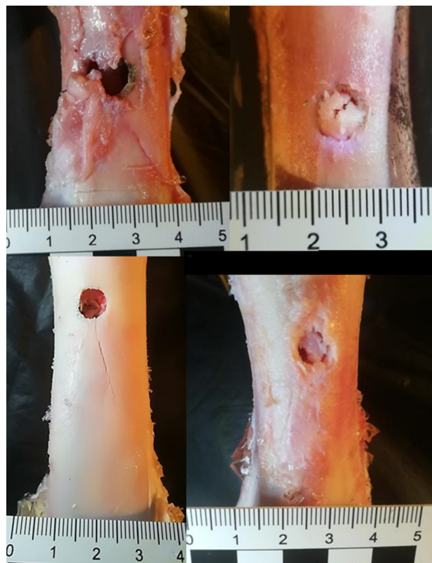
Fig. 17. Inlet damage to the anterior surface of the femoral shaft using 6.35 mm caliber shot. From the top, left H&N Baracuda, right H&N Hollowpoint; from the bottom, left H&N Spitzkugel, right Black Max Lead-Free
