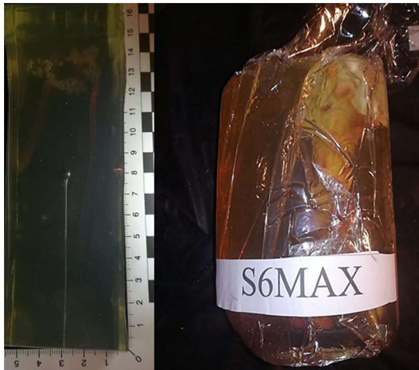
Fig. 12. The result of a sample calibration test of ballistic gelatin (left), and a finished model with coding (right)
