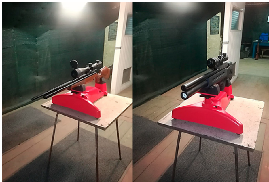
Fig. 10. Air Arms S410 Xtra FAC cal. 5.5 mm (pictured left) and FX Bobcat Mk II cal. 6.35 mm (pictured right) air carbines on a Predator PSR-30MTM stand
